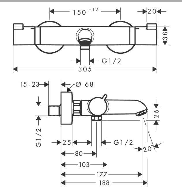
**Ecostat Comfort****Thermostatique bain/douche apparent**Finition: **Chrome** N° Art.: **13114000**
